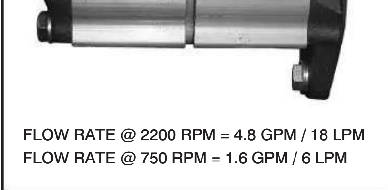
Illustration 22-11. Auxiliary Pump
