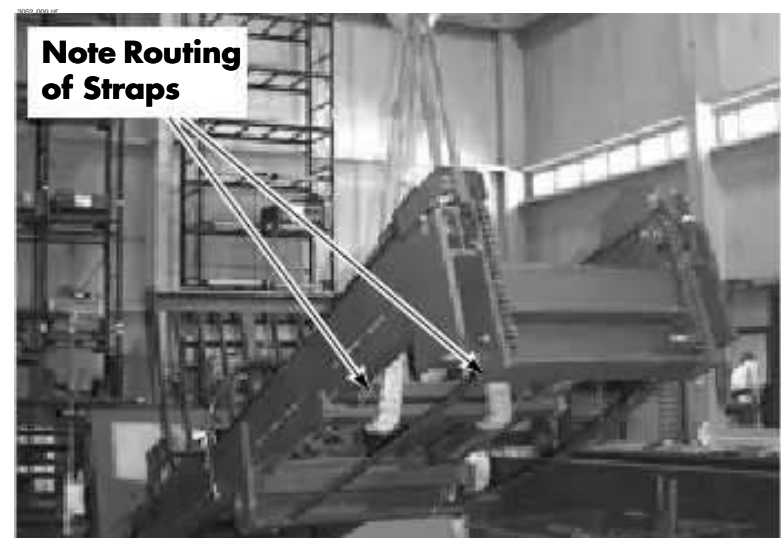
Figure 3-4. 9700 Mast Strapped to Hoist
