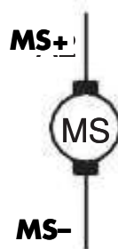
Figure 5-2. Permanent Magnet Motor Circuit
