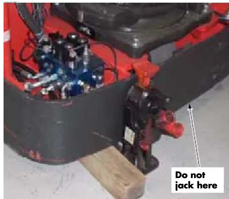
Figure 2-5. Jacking and Blocking Tractor
