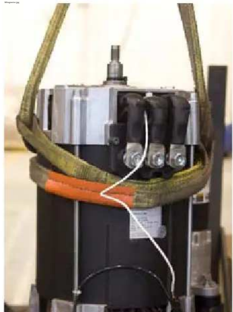
Figure 2-8. Lifting Traction Motor
