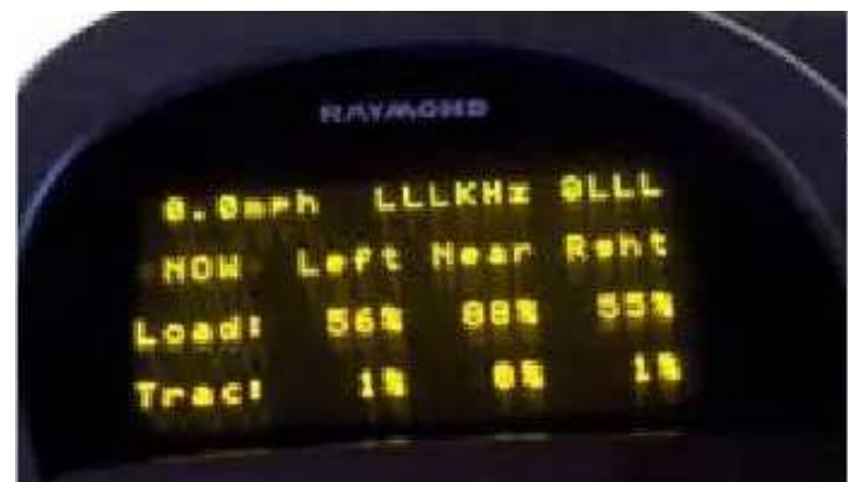
Figure 5-10. Coil Readings - Bad Tractor Antenna
