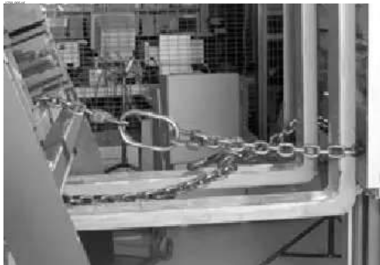
Figure 3-2. 9600 Mast Erection, Alternate Method
