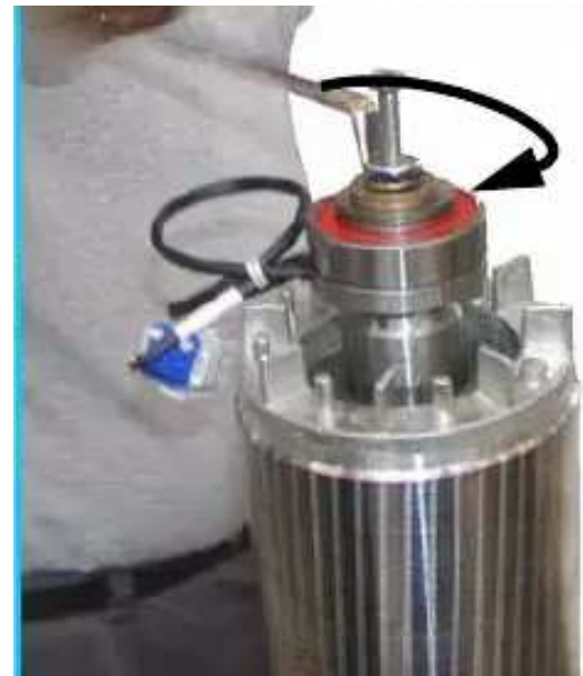
Figure 7-48. Driving Encoder Onto Motor Shaft
