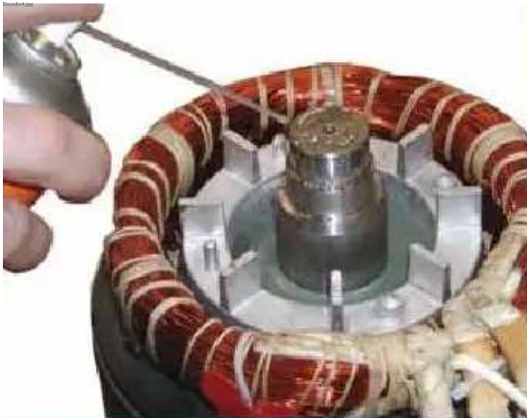
Figure 7-46. Lubricate Motor Shaft
