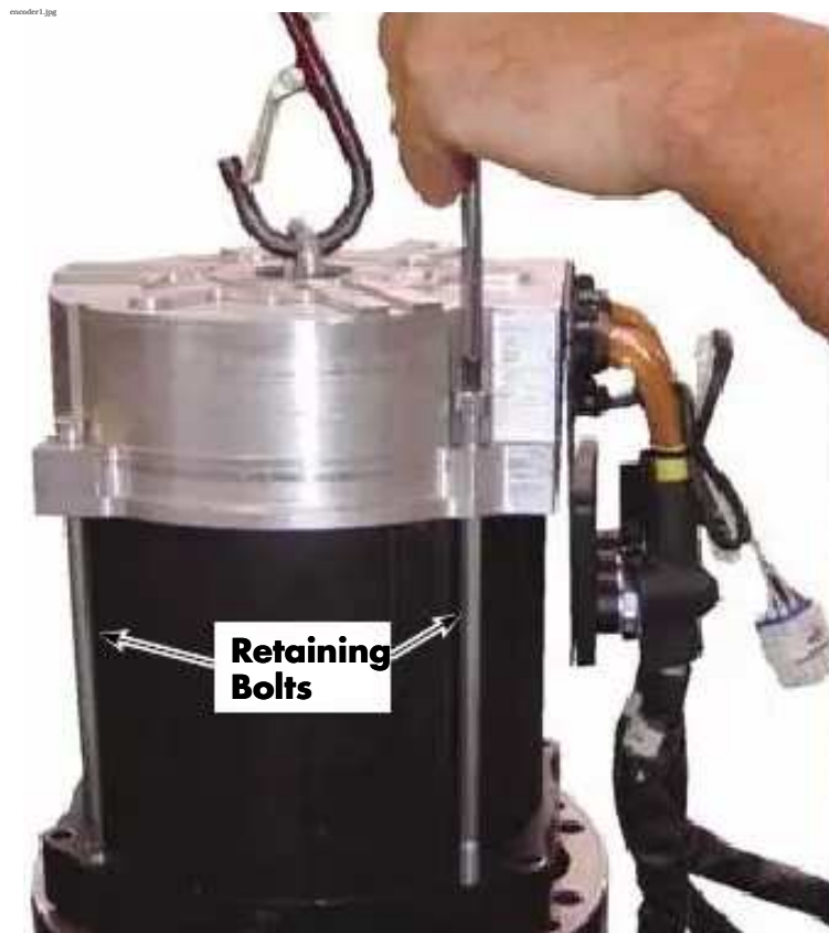
Figure 7-43. Retaining Bolt Removal
