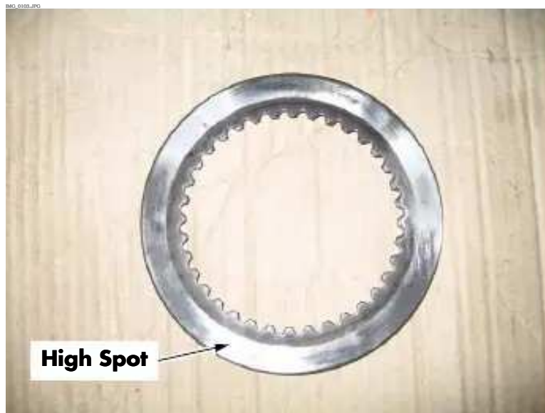
Figure 7-12. High Spots On Brake Disk
