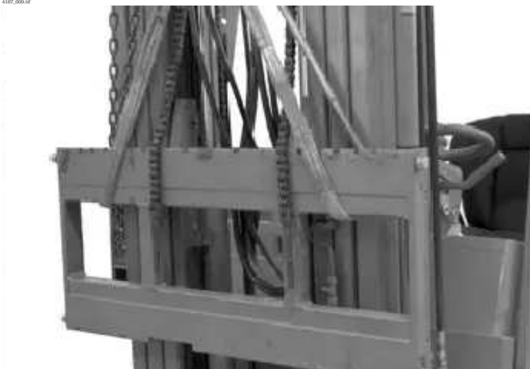
Figure 7-59. Secure Carriage to Hoist
