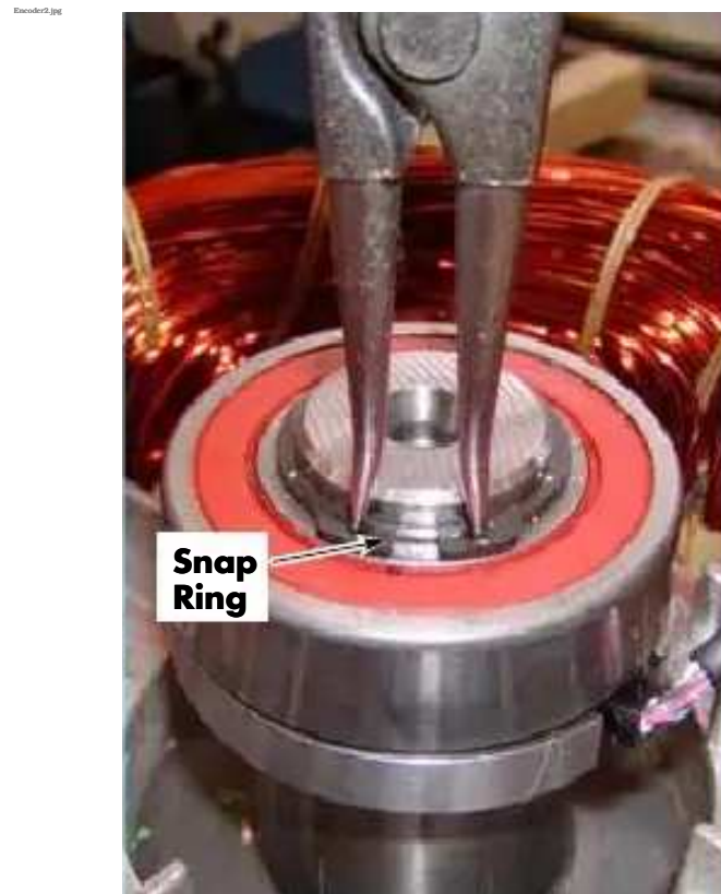
Figure 7-44. Snap Ring Removal
