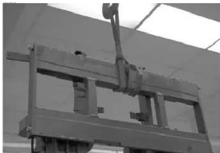
Figure 7-60. Carriage Removal/Installation Through Top of Mast
