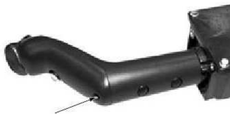
Figure 7-11. Cover Retaining Screw - Top
