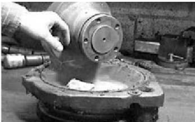
Figure 7-26. Inspect Housing for Hub Wear
