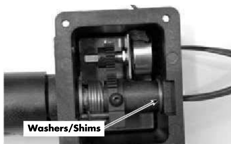
Figure 7-18. Travel Pot/Bracket Assembly Installation
