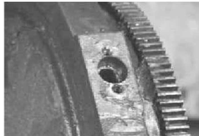
Figure 7-101. Remove Steel Ball Bearings
