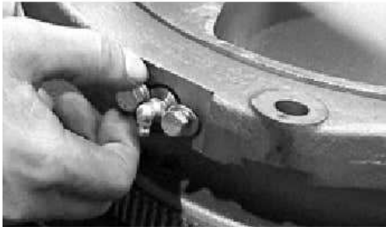
Figure 7-96. Filler Plug Bolt Installation
