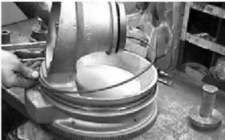
Figure 7-92. Radial Ring Installation on Housing
