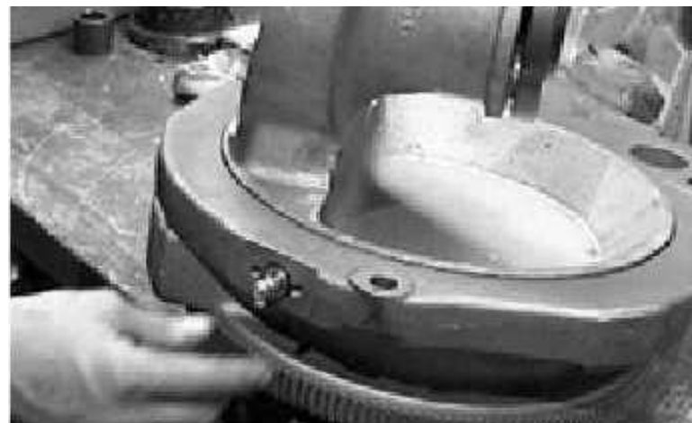
Figure 7-95. Bearing Filler Plug Installation
