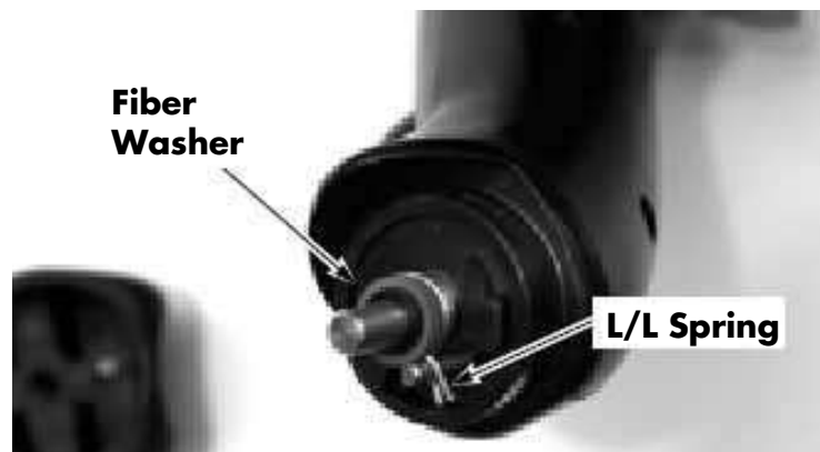
Figure 7-9. Spacer Washer and L/L Spring Removal
