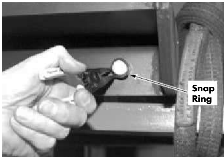
Figure 7-182. Snap Ring, Pivot Pin, and Mounting Block
