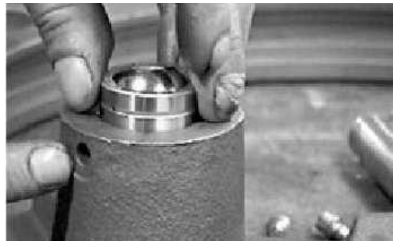
Figure 7-86. Spherical Bearing Alignment
