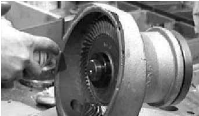
Figure 7-97. Apply Gasket Compound
