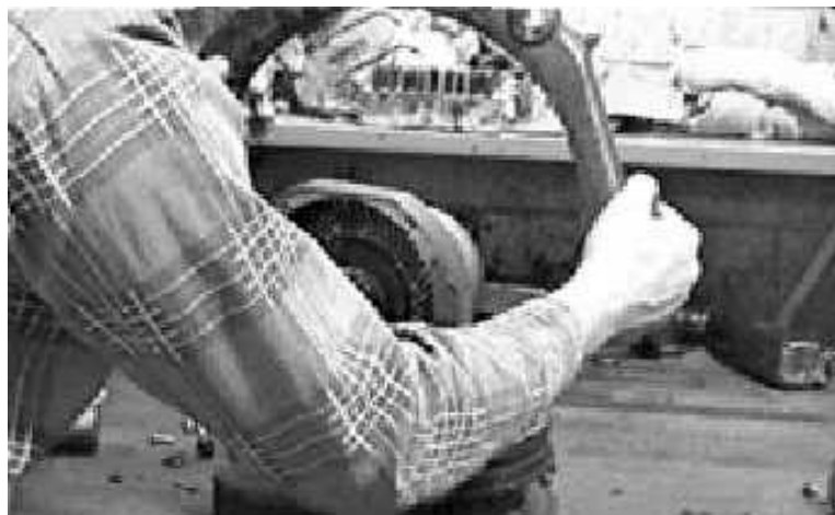
Figure 7-29. Pivot Ring Removal
