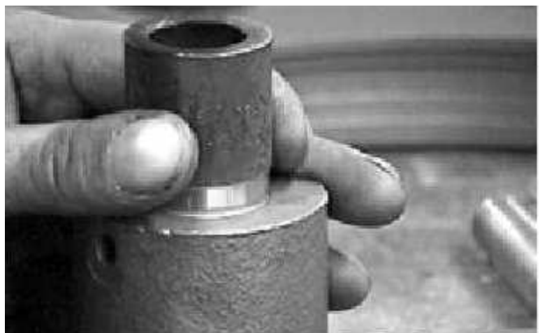
Figure 7-87. Install Spherical Bearing
