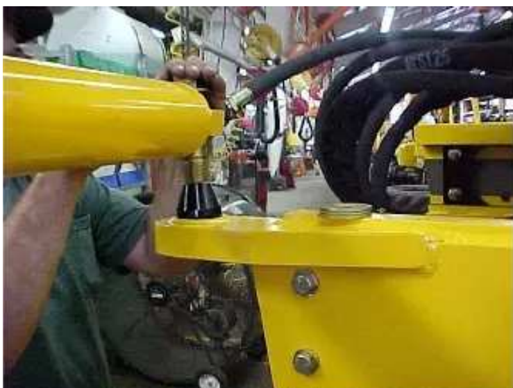
LINING UP THE CYLINDER, MOUNTING CONE, AND BOLT.
