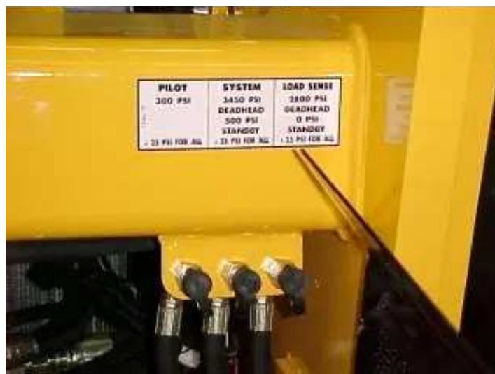
Pressure Checks, Valve in Back
