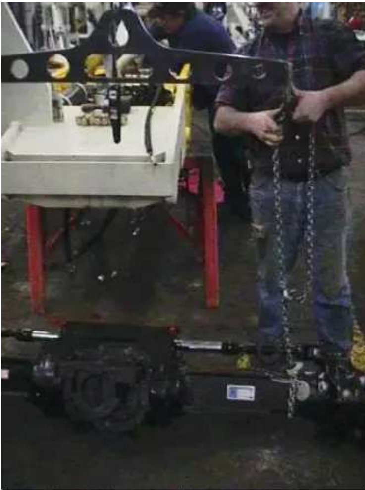
ATTACHING SLING AND CHAINS LIFTING AXLE
