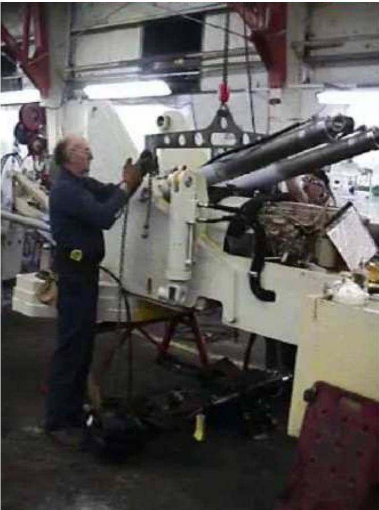
ATTACHING SLING AND CHAINS LIFTING AXLE
