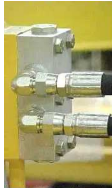
CONNECT HYDRAULIC LINES TO CYLINDER
