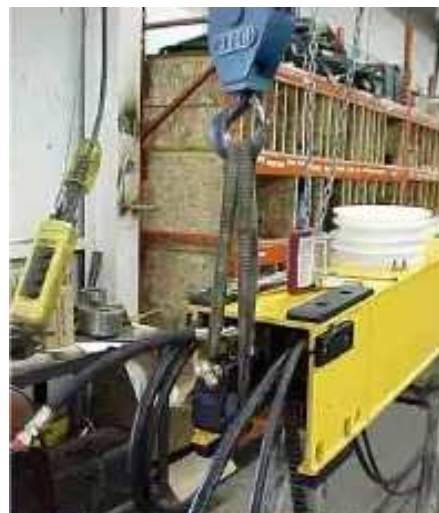
24. The extend cylinder is fully into the boom at this point. Before installing the pin, shine a light through the tip end of the boom to check alignment of the cylinder. Install pin through extend cylinder and attach with locktight and bolt. Attach boom length decal to middle boom.
