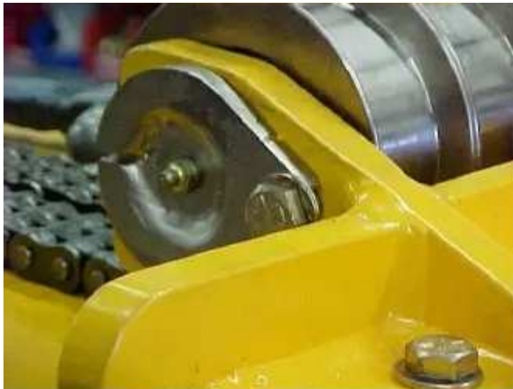
20. Install the extend cylinder grease fitting and move hoses and chain to ease in installation.
