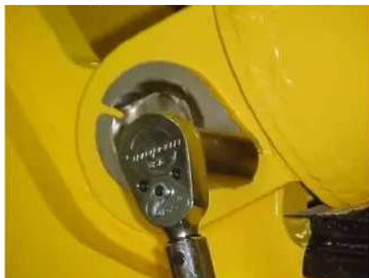
TORQUE CAPSCREW TO PROPER SPECIFICATION.
