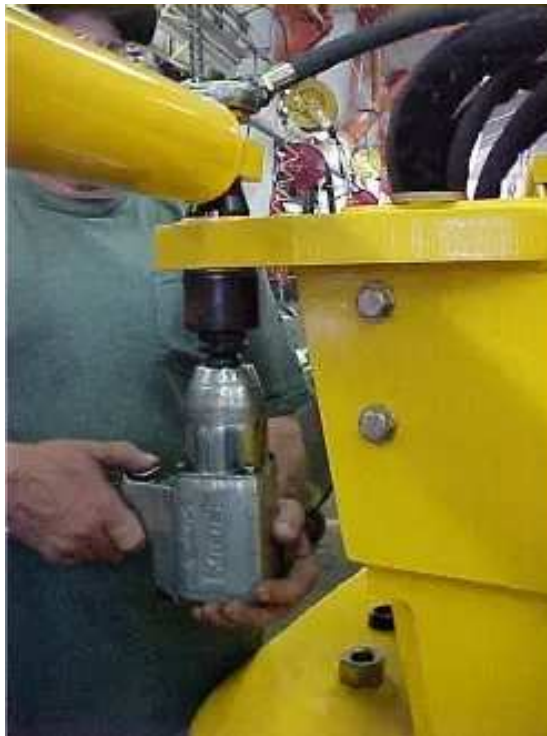
TIGHTENING REAR BOLT.
