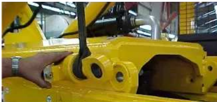
RE-LOCATION OF LIFTING STRAP AND LINING UP OF THE FRONT MOUNT.
