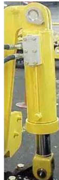
FULLY INSTALLED SWAY CYLINDER
