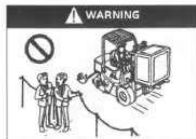
People are not allowed to start in work place!
