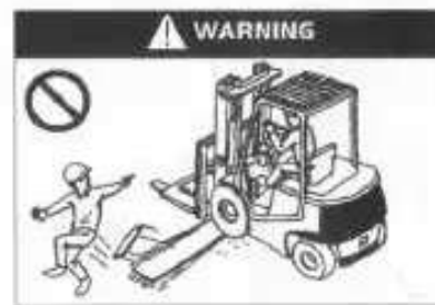
Prohibit crossing the obstacle such as a trench, mound and railway!
