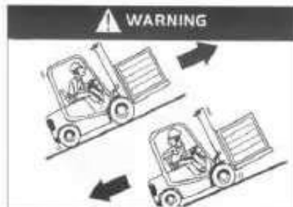
when loading,travel forward in upgrade and backward in downgrade
