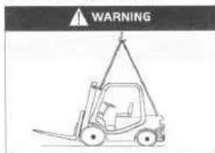
Hoisting the forklift correctly!
