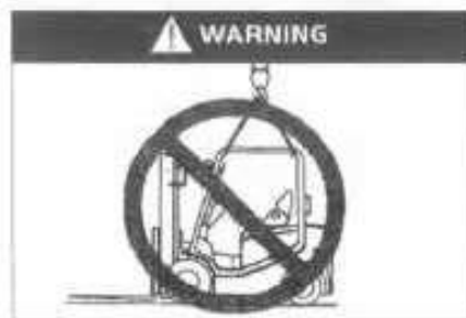
Forbid hoisting from the top!
