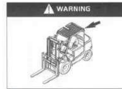
Do not move the overhead guard!
