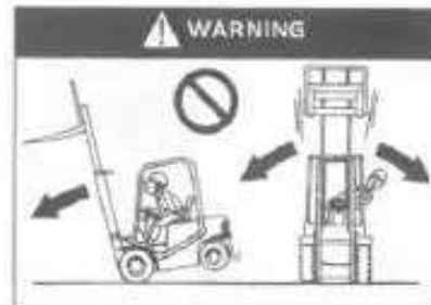
When moving, the distance between fork and ground should be less than 150mm to 200mm!
