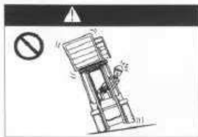
When the truck is not in the horizontal position, do not load or unload!
