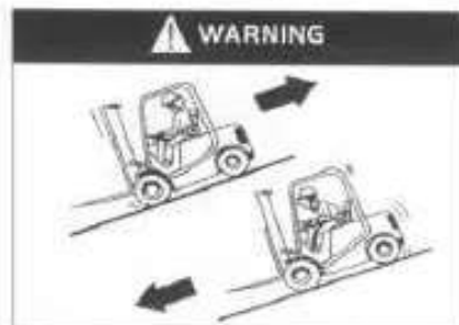
When no-load,travel backward in upgrade and travel forward in downgrade!
