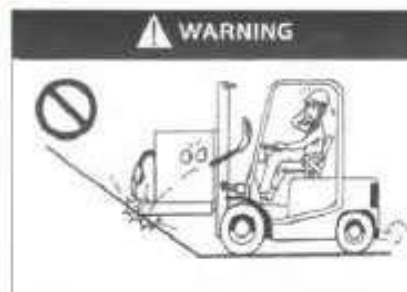
Pay attention to the steep uphill slopes and goods lifting height!
