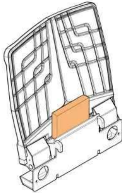
Figure 29. Supporting the operator's platform during installation
