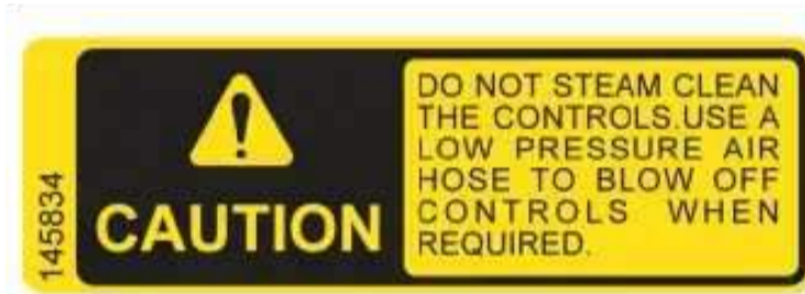
Figure 114. Electric panel cleanup warning sticker
