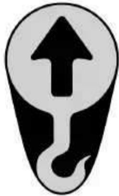
Figure 116. Hoist point indication sticker
