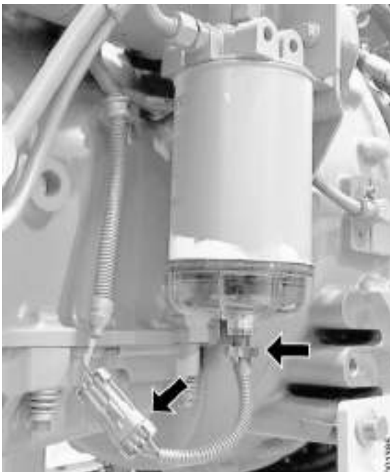
Fuel pre-filter, drain valve and connector for water in fuel sensor
