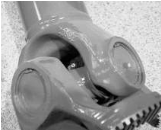
Grease nipple for universal joint, example
