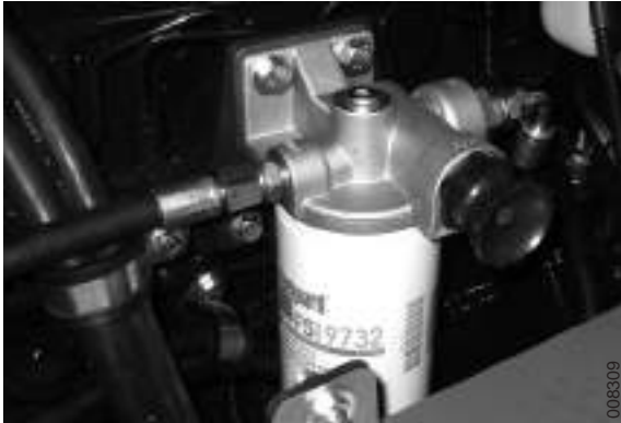
Fuel hoses on fuel filter
