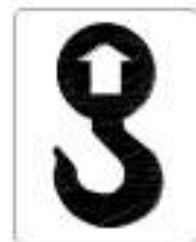
22. hang label: show the hang position. When hanging, the rope should not touch the light and even destroy it.
