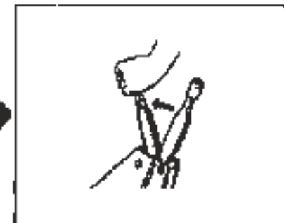
Push the parking brake lever
