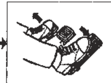
Gradually depress the accelerator pedal while releasing the inching pedal.
