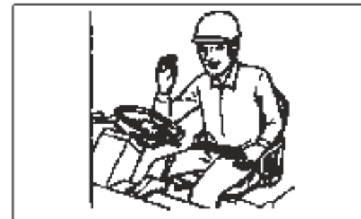
Be sure to fasten the seat belt before operating the truck. Remember, the belt will not restrain you in an accident if it is not fastened properly.
