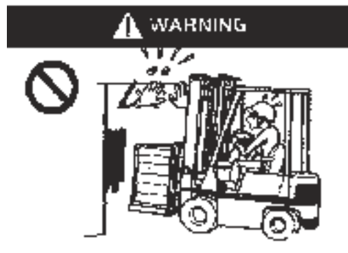
Always check overhead clearance!
