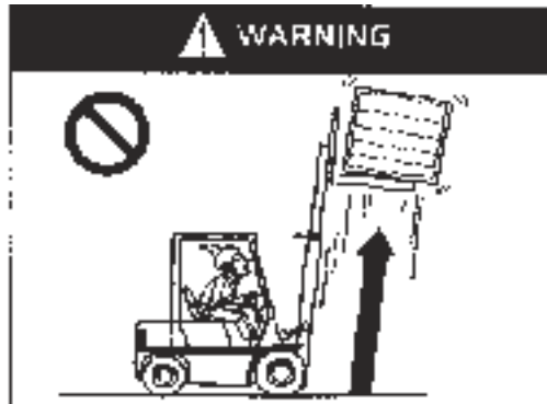
DO NOT elevate tilted loads!
