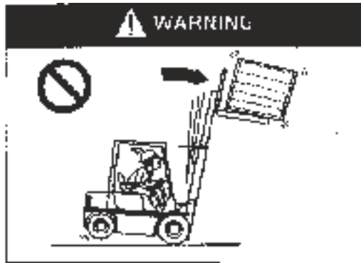
DO NOT tilt elevated loads forward!
