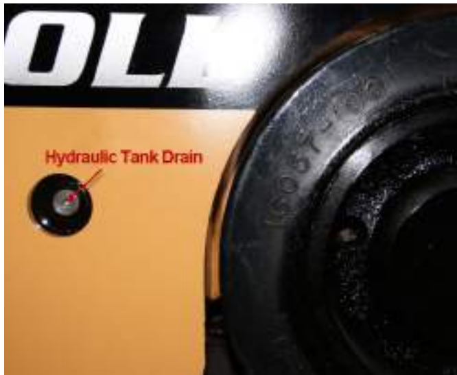
Figure 3-1: Hydraulic Tank Drain
