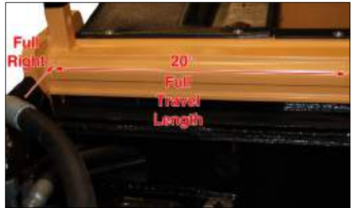
Figure 6-17 Marking the Frame
