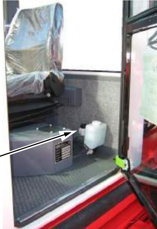
Hydraulic oil tank of pedal compensation system
