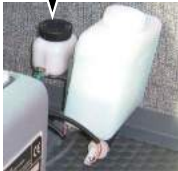
Hydraulic oil tank of pedal compensation system
