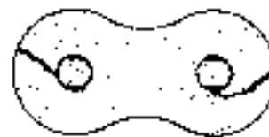
Corroded Chain (with Stress-Corrosion Cracks)
