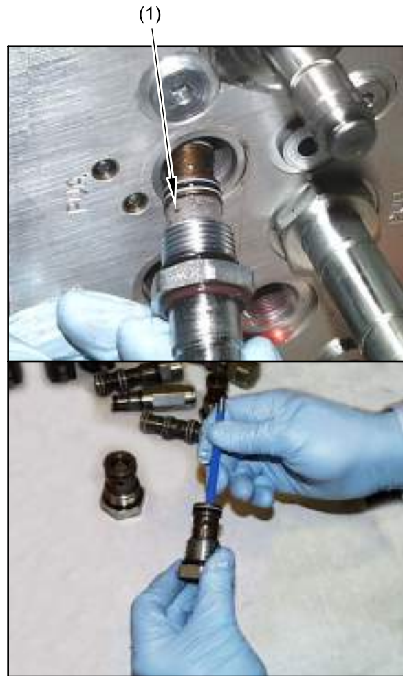
(1) Note visible contamination on valve screen
