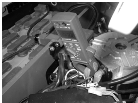
Measuring method Procedure using a clamp amperometer
