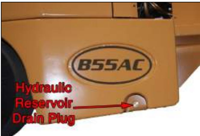
Figure 3-7: Hydraulic Oil Drain Plug
