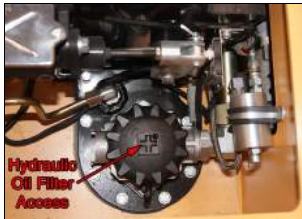
Figure 3-8: Hydraulic Oil Filter Cap
