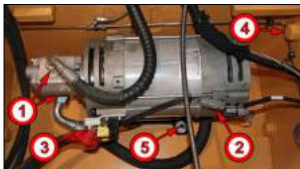
Figure 3-10: Hydraulic Pump Removal
