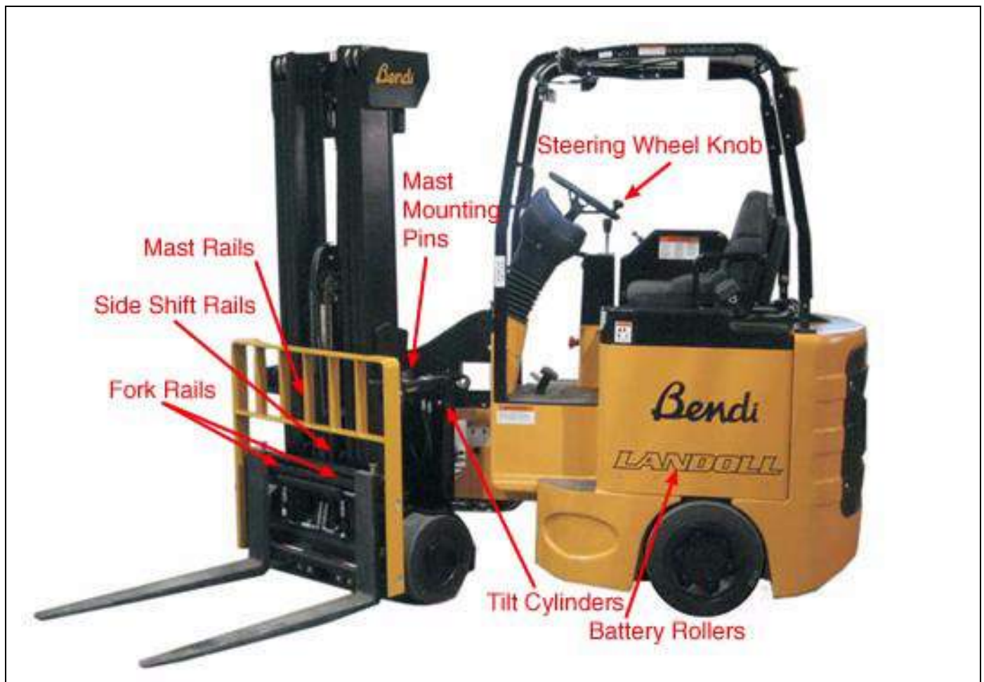
Figure 1-2: Lubrication Locations
