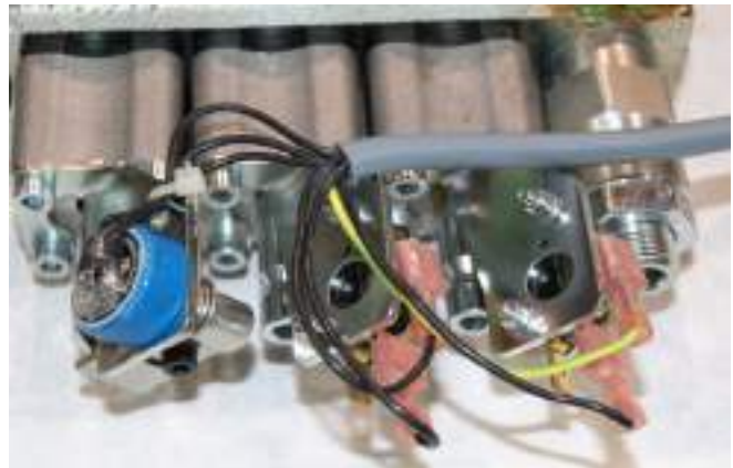
Figure 3-5 Hydraulic Valve Switches
