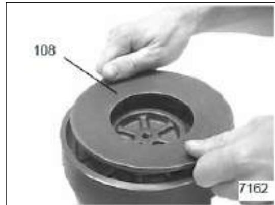
Figure 3-54: Install Spring Washer
