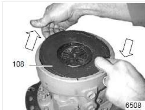
Figure 3-57: Remove Spring Washer
