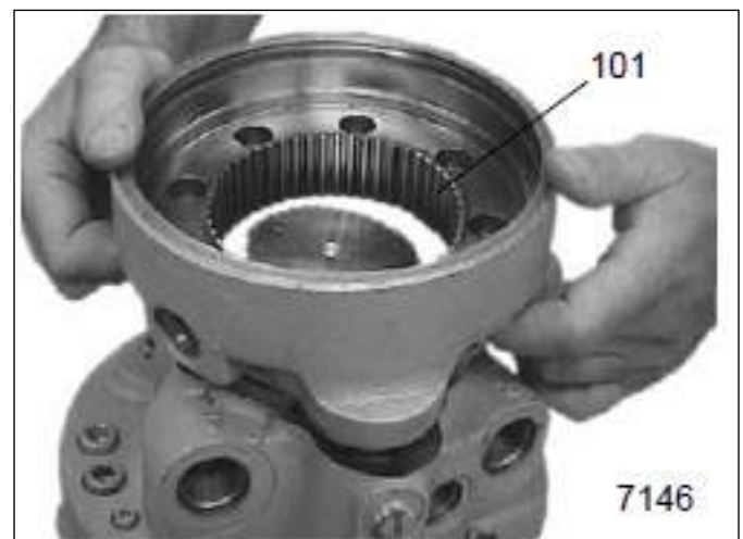
Figure 3-36: Remove Brake Housing
