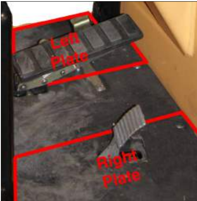
Figure 2-26: Floor Plate Removal
