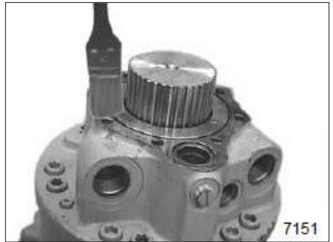
Figure 3-42: Brush Loctite on Valve Cover Surface
