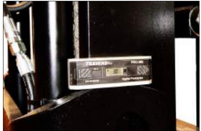
Figure 2-13: Tilt Gauge Placement
