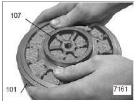
Figure 3-53: Install Brake Piston
