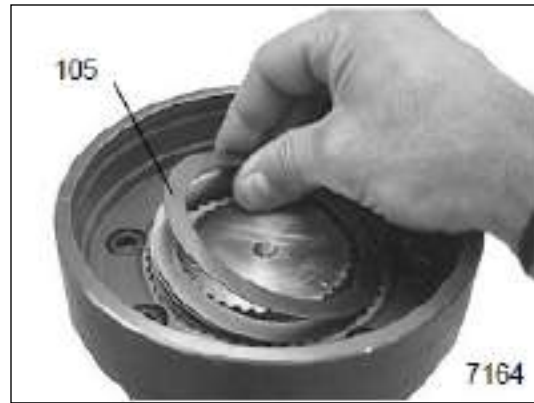
Figure 3-59: Install Shims on Last Disc, Thickest First
