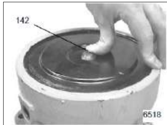
Figure 3-65: Install New Plug
