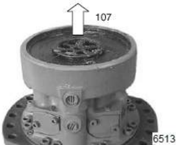
Figure 3-33: Remove Brake Piston
