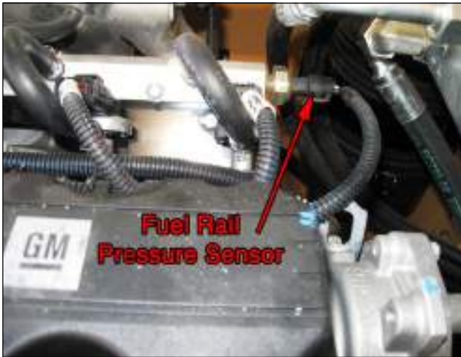
Figure 5-9: Fuel Pressure Sensor Location
