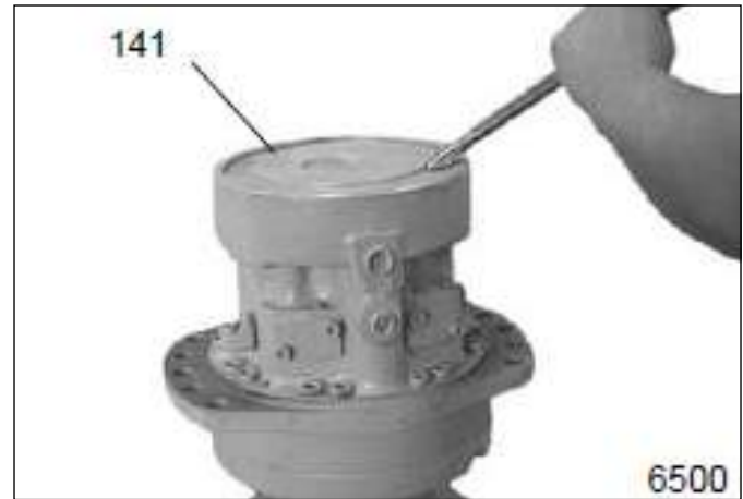
Figure 3-29: Remove Brake Cover
