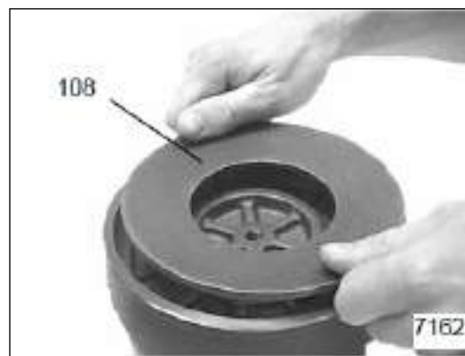
Figure 3-60: Reinstall Brake Piston and Spring Washer
