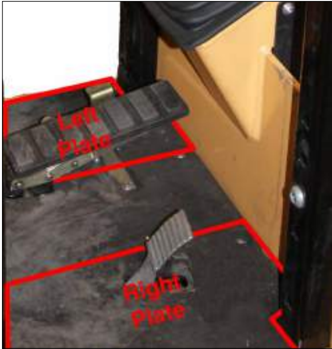
Figure 3-1: Floor Plate Removal
