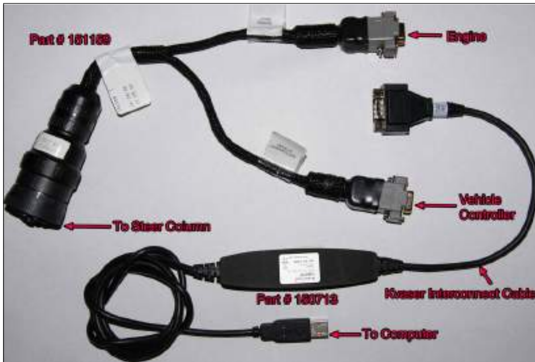
Figure 4-2: Computer Interface Cables
