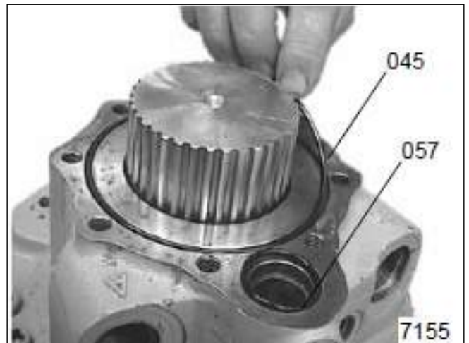
Figure 3-43: Install New O-Ring
