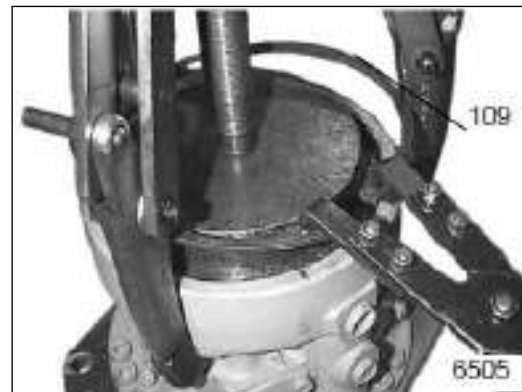
Figure 3-55: Apply 15,740 lbs to Snap Ring
