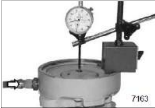
Figure 3-56: Measure P Brake Piston Stroke with Dial Gauge
