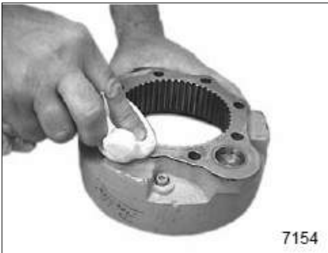
Figure 3-41: Wipe Brake Housing with Moist Cloth, Inside to Outside
