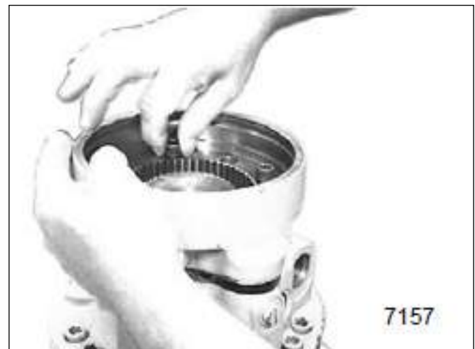
Figure 3-46: Position by Hand Tightening Bolts
