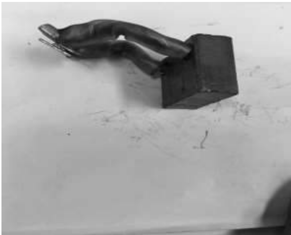
3. With a phillips screwdriver unscrewed the screw, can take out the carbon brush, for replacement. The installation process is the process of inverse process
