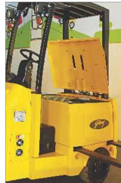
Fork pockets for easy removal of battery
