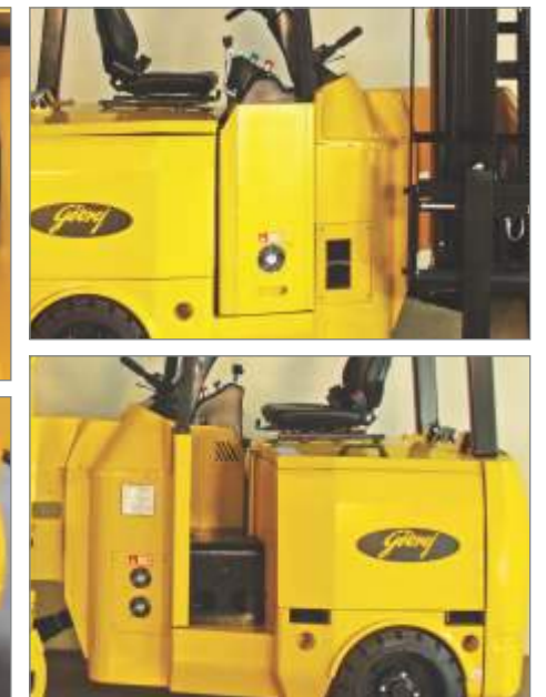
Single allen key required to access control units
