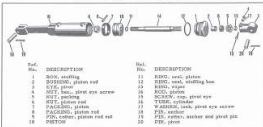
Fig. 17. Tilt Cylinder and Mounting (New Type)
