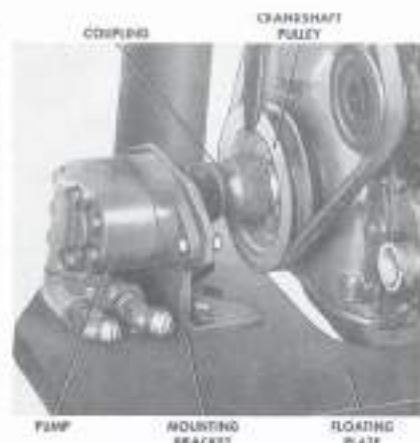
Fig. 11. Hydraulic Pump - Installed View
