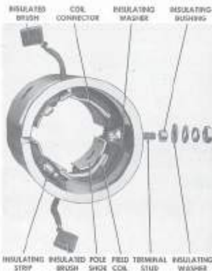
Fig. 45. Field Coil Insulation
