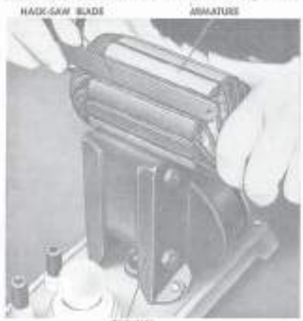
Fig. 28. Testing Armature in a Growler
