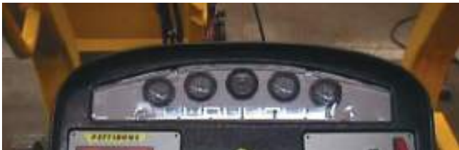
Figure 17. Gauges as pictured left to right: Transmission Oil Pressure, Transmission Temperature, Hour Meter, Coolant Temperature, Fuel Gauge
