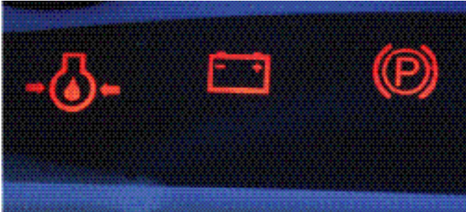
Figure 18. Warning Lights as pictured left to right: Oil Pressure, Low Battery, Parking Brake
