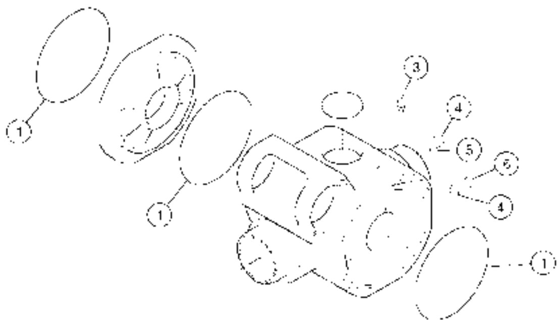
**AXLE 4-WHEEL DRIVE STEERING (59251662) - INTERNAL BREAKDOWN**
