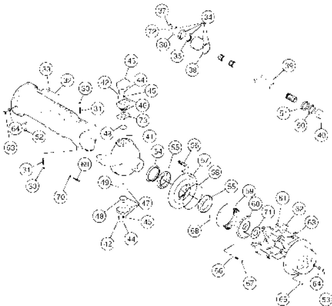
**AXLE 4-WHEEL DRIVE STEERING (59251662) - INTERNAL BREAKDOWN**
