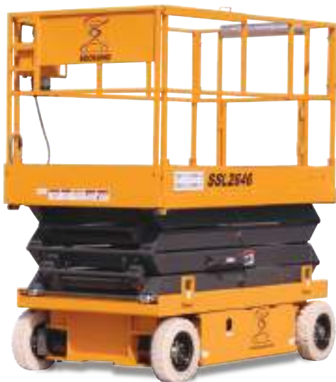
◀ SSL-2646 Max. Platform Height 7.9M (Max. Working Height 9.9M)
