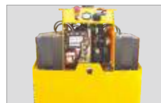
MOSFET Control System
