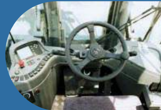
A comfortable and intelligently designed cabin with a new instrument panel, not only makes forklift operators happier, it makes them more productive as well. The seat, steering column and operating controls are all adjustable to suit individual preferences. (The cabin is equipped with optional display and electro hydraulic levers.)
