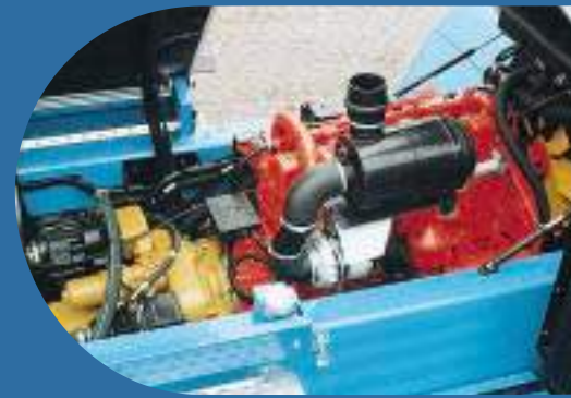
Excellent accessibility for servicing. The cabin hydraulically tilts to the side and the engine cover can easily be lifted to expose the entire drive train and hydraulic components.
