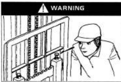
Check the position of fork dowl pin!
