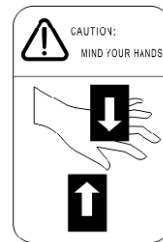
"Squeezing Alarm" Label
