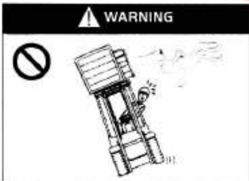
No lifting when it is too windy!
