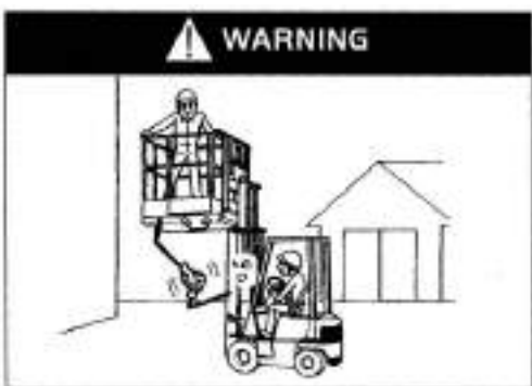
Use safety equipment to lift people for work at heights!
