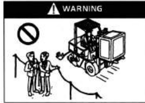
No passing through the working area!
