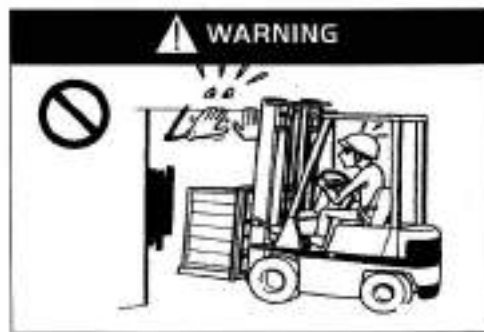
Pay attention to the height for working area!
