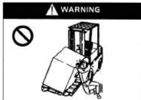
Do not carry the damaged package on shoulder!
