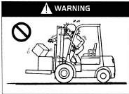
Do not stretch out from the machine during driving!
