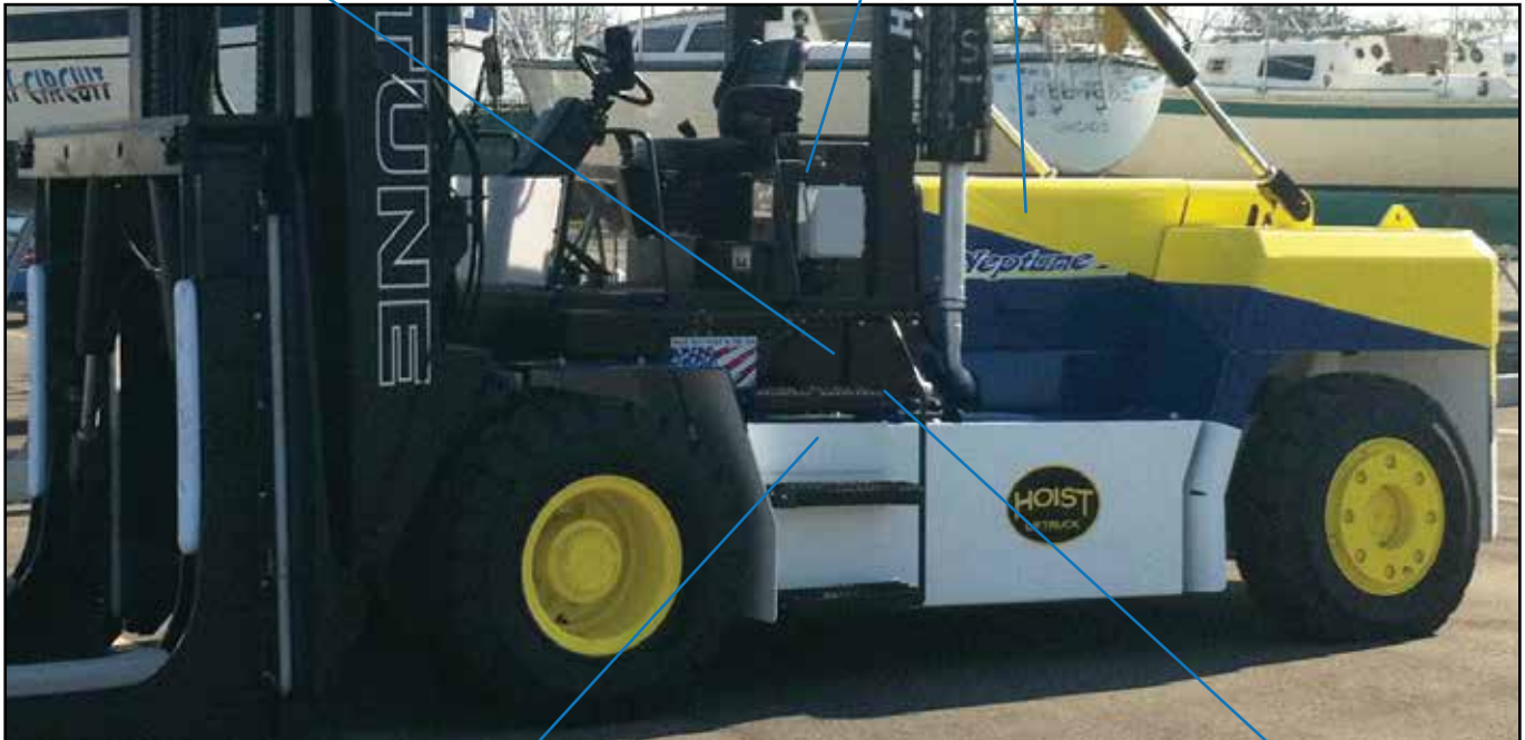
Located on both sides of the forklift, flip-open panels allow quick and easy access to the complete drive line, batteries and hydraulic multi-gauge.
