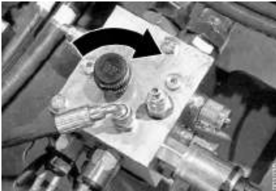
Adjusting screw accumulator charging pressure
