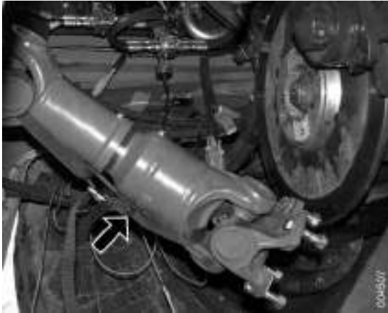
Securing propeller shaft.
