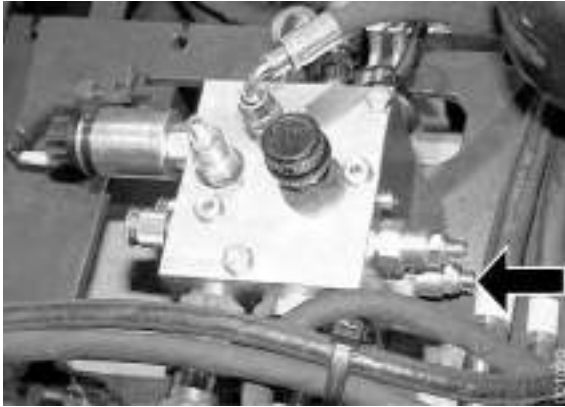
Adjusting screw accumulator charging pressure
