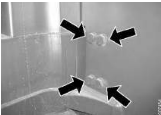
Attaching bolts steering cylinder.
