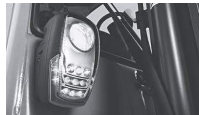
External LED lighting for excellent light conditions
